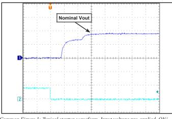
Common Figure 1: Typical startup waveform. Input voltage pre-applied, ON/ OFF Pin on Ch 2. Output voltage normalized.
