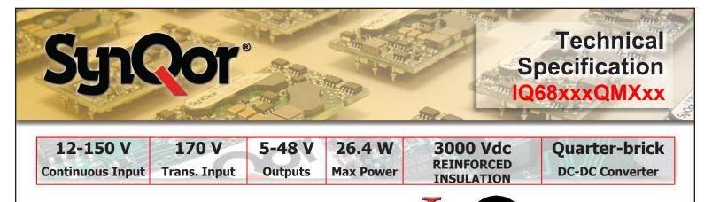
The InQor<sup>®</sup> Quarter-brick converter series is composed of next-generation, board-mountable, REINFORCED INSULATED, fixed switching frequency dc-dc converters that use synchronous rectification to achieve extremely high power conversion efficiency. Each module is supplied completely encased to provide protection from the harsh environments seen in many industrial and transportation applications.
