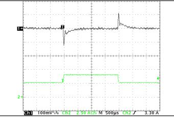
Figure 5: Output voltage response to step-change in load current (50 % -75 % -50 % of lout(max); dI/dt = 0.05 A/ $\mu$ s. Load cap: 15  $\mu$ F tantalum cap and 1  $\mu$ F ceramic cap. Ch 1: Vout, Ch 2: lout.
