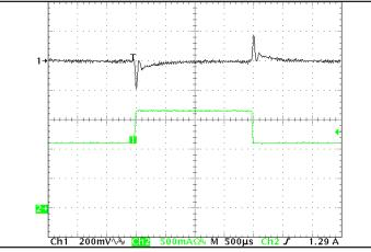
Figure 5: Output voltage response to step-change in load current (50 % -75 % -50 % of lout(max); dI/dt = 0.03 A/ $\mu$ s. Load cap: 15  $\mu$ F tantalum cap and 1  $\mu$ F ceramic cap. Ch 1: Vout, Ch 2: lout.
