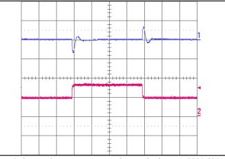
Figure 5: Output voltage response to step-change in load current (50 % -75 % -50 % of Iout(max); dI/dt = 0.02 A/µs. Load cap: 1 µF ceramic cap. Ch 1: Vout (1 V/div), Ch 2: Iout (500 mA/div), time scale: 500 µs/div.
