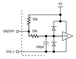
Figure B: Internal ON/OFF pin circuitry
