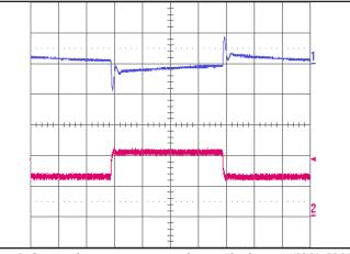
Figure 5: Output voltage response to step-change in load current (50 % -75 % -50 % of Iout(max); dI/dt = 0.01 A/µs. Load cap: 1 µF ceramic cap. Ch 1: Vout (1 V/div), Ch 2: Iout (200 mA/div), time scale: 500 µs/div.
