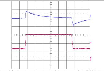
Figure 6: Output voltage response to step-change in input voltage (600 V/ms), at Max. load current. Load cap: 1  $\mu$ F ceramic cap. Ch 1: Vout (2 V/div), Ch 2: Vin (50 V/div), time scale: 1 ms/div.
